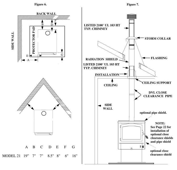
**NOTE:** All clearances are to combustibles with optional close clearance shields and pipe shield, using DVL Close Clearance pipe, and minimum floor protector.
