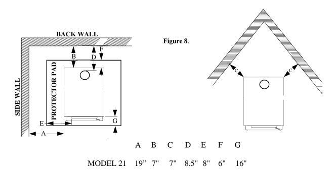
**NOTE:** All clearances are to combustibles with close clearance shields and pipe shield, DVL Close Clearance pipe with elbow and minimum floor protector.
