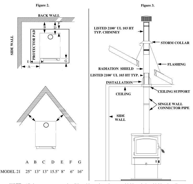
**NOTE:** All clearances are to combustibles without close clearance shields and pipe shield, using 6" Single Wall minimum 24 ga. blued or black pipe and minimum floor protector. The clearances above may be reduced. Follow **NFPA-211** codes if available or follow instructions on (Pages 10, and 11).
