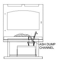
OPEN MAIN DOOR TO FIRE BOX. LOCATE ASH DUMP TOP LID IN RIGHT REAR OF HEATER. OPEN ASH DUMP TOP LID AND SWEEP ASHES INTO ASH DUMP CHANNEL. **(4)**
