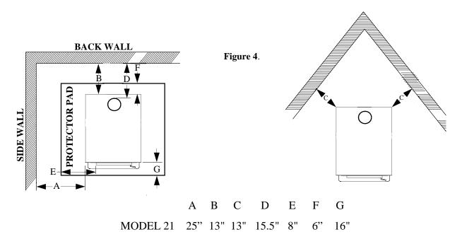
**NOTE:** All clearances are to combustibles without close clearance shields and pipe shield, 6" Single Wall minimum 24 ga. blued or black pipe with elbow and minimum floor protector. Clearances above may be reduced. Follow **NFPA-211** codes if available or follow instructions on (Pages 12, and 13).
