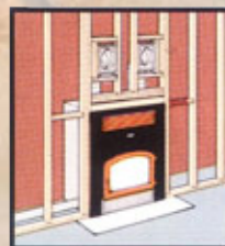
Assemble hot air ducts and frame in fireplace.
