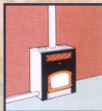
Place fireplace and install combustion air duct and chimney.
